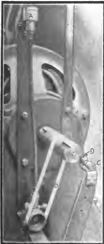
Fig. 5—Free end of armature shaft with tachometer A operated by belt B and counter C connected with or disconnected from shaft by trigger D
